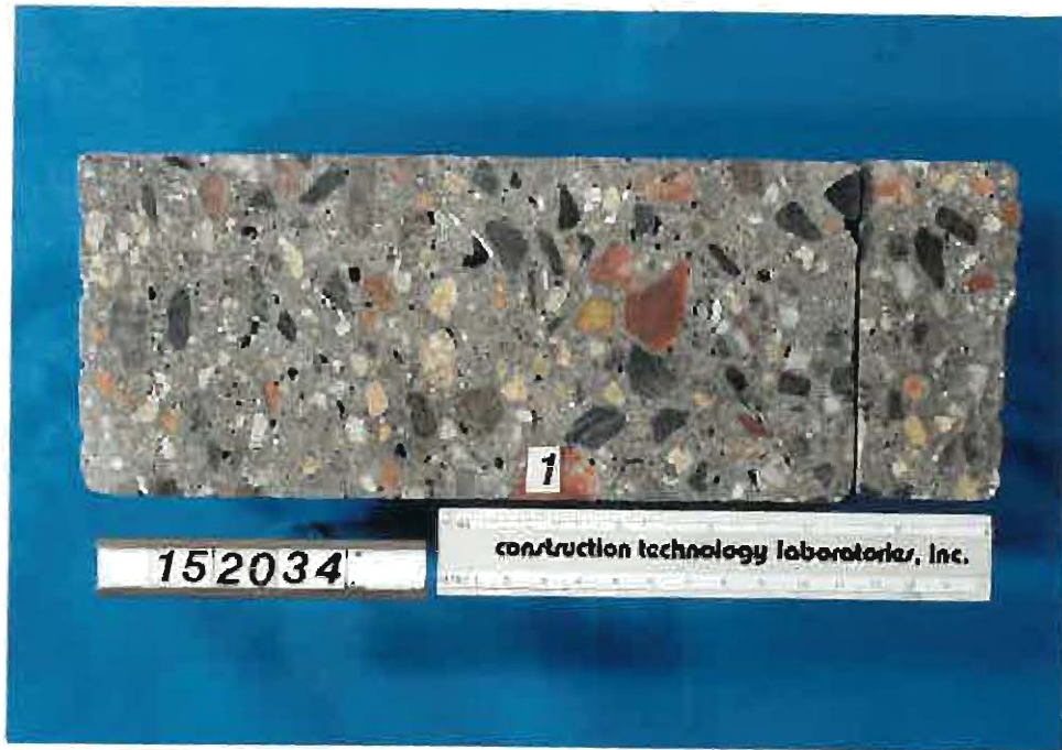
FIG. 3 LONGITUDINALLY SAWED AND LAPPED SLICE OF CORE NO. 1 SHOWING 1/2 INCH CRUSHED STONE AND 3/8-INCH PEA GRAVEL COARSE AGGREGATES. CORE WAS SAWCUT NEAR BOTTOM SURFACE TO FIT INTO LAPPING MACHINE.
