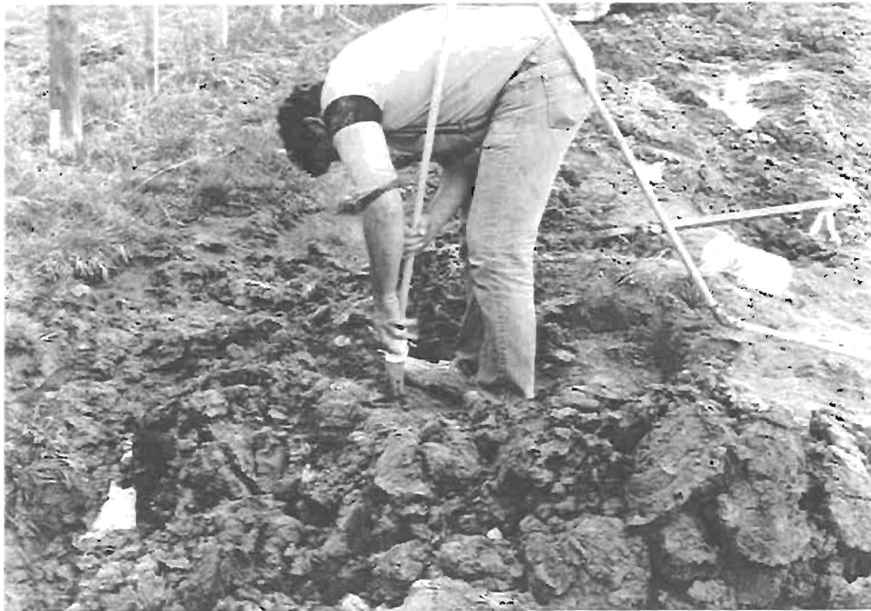
Figure 16 Water sometimes got into the tube. This made it necessary to extract the water from the tube as is being done in this photo.
