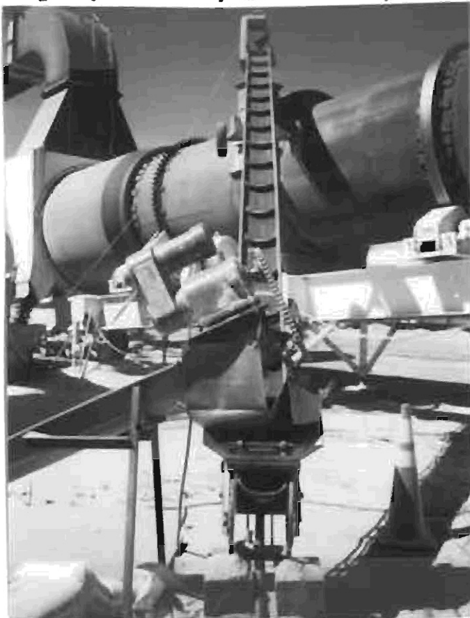
Figure 9. Conveyor System Used to Add Vestoplast S and Fiber Pellets at the RAP Collar.
