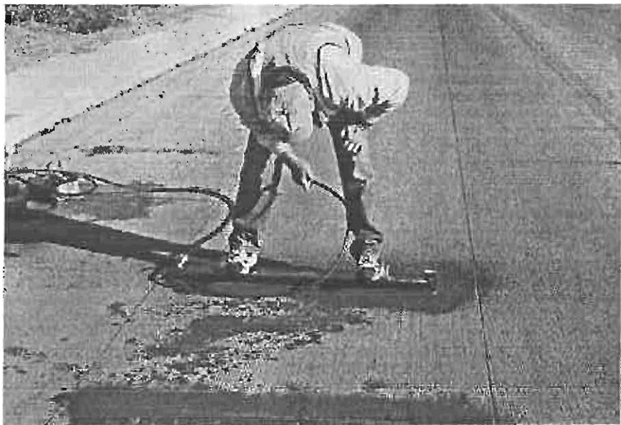
Figure 6 The operator stands on the test chamber to help seal it to the pavement surface. The vacuum level in the chamber can be regulated by opening and closing the end of the hose.
