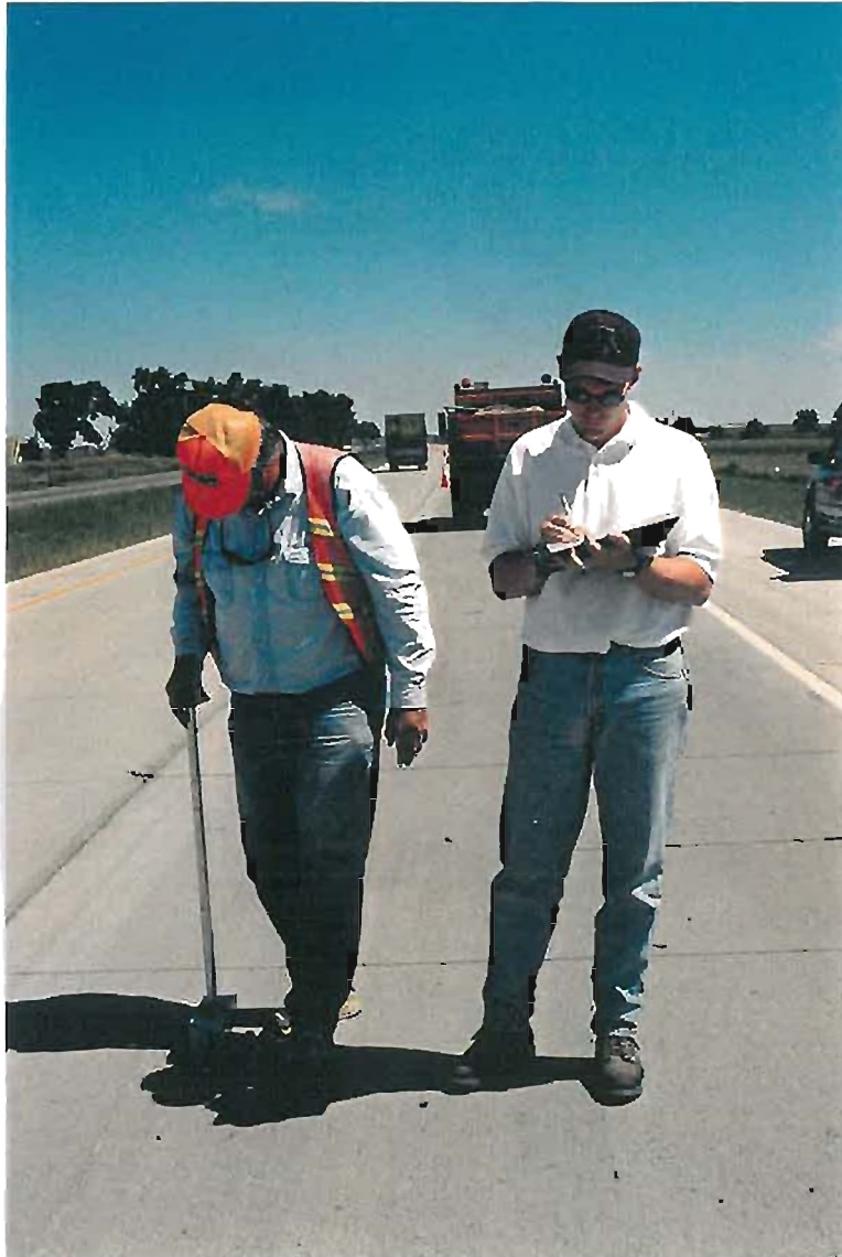
Figure B.13 - Collecting Profile Elevation Measurements Using the Dipstick at CDOT Project #2
