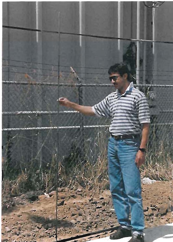
Figure A.6 - Typical Invar Rod Used for Profile Elevation Reference Prior to Embedment
