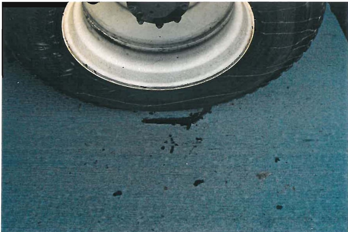
Figure B.12 - Typical Placement of Truck Tires Adjacent to Strain Gages for Load Testing
