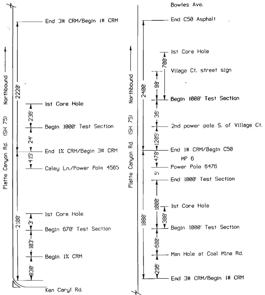
**Figure 2. Location of Crumb Rubber Sections.**
