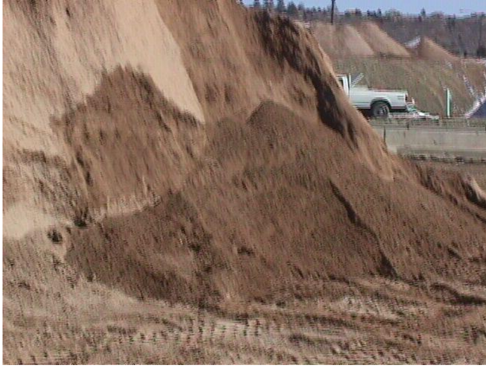
Figure B-5. Backfill material meeting requirements for CDOT Class 1 backfill.
