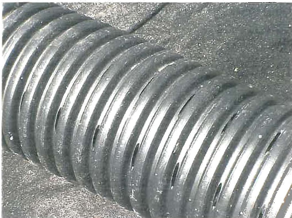
Figure 15. Close-up of perforated drainpipe & geotextile.
