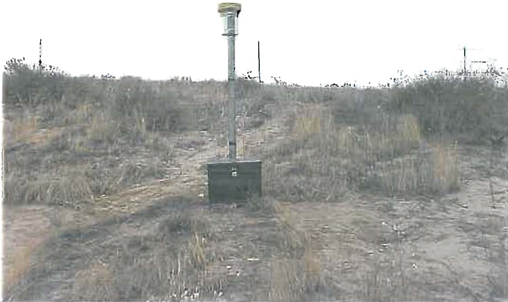
Figure 20. ATE 525WS rain gauge with 8-inch collector.
