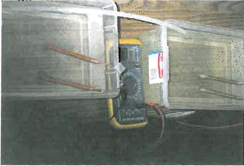
Figure 34: The corrosion potential test unit for copper components.
