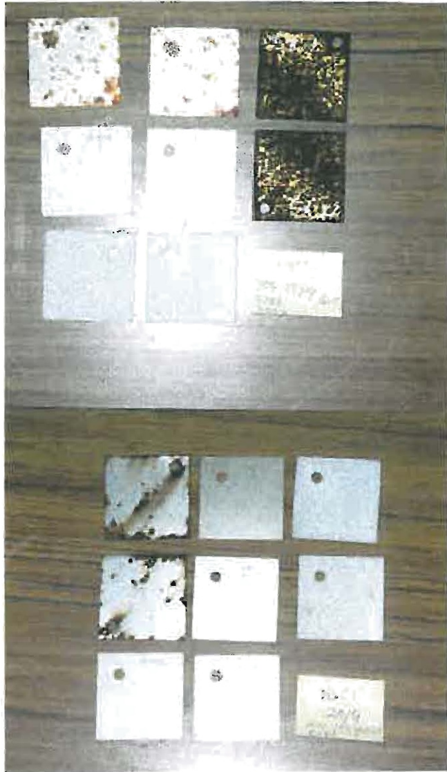
Figure 30: The coupons after the cyclic exposure test for one and half a month with reagents.
