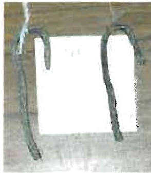
Figure 14c: Corroded copper wires after SAE J2334 testing
