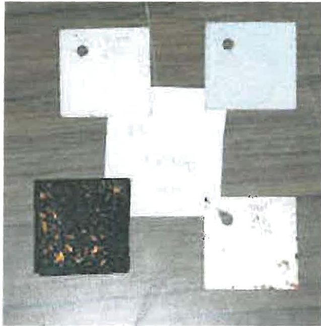
Figure 32: The coupons after the cyclic exposure test for two months with \text{NaCl} + \text{MgCl}_2 .
