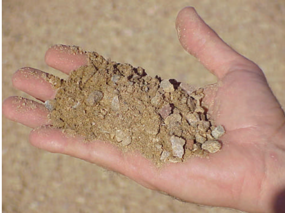
A current sample of coarse crushed aggregate from the same gravel source used in the I-25 construction.
