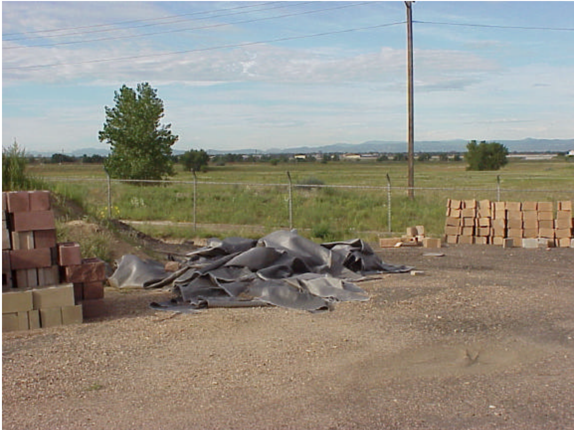
Photo 13. Retrieved Geotextile Sheets and Whole Blocks from the Structures.
