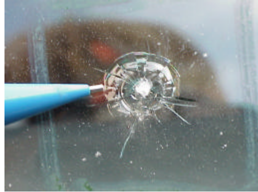
Figure 8.3.4 Radial Crack Fracture "Star" from Particle Impact
