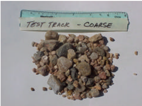
Fig 3 Coarse road test gravel
