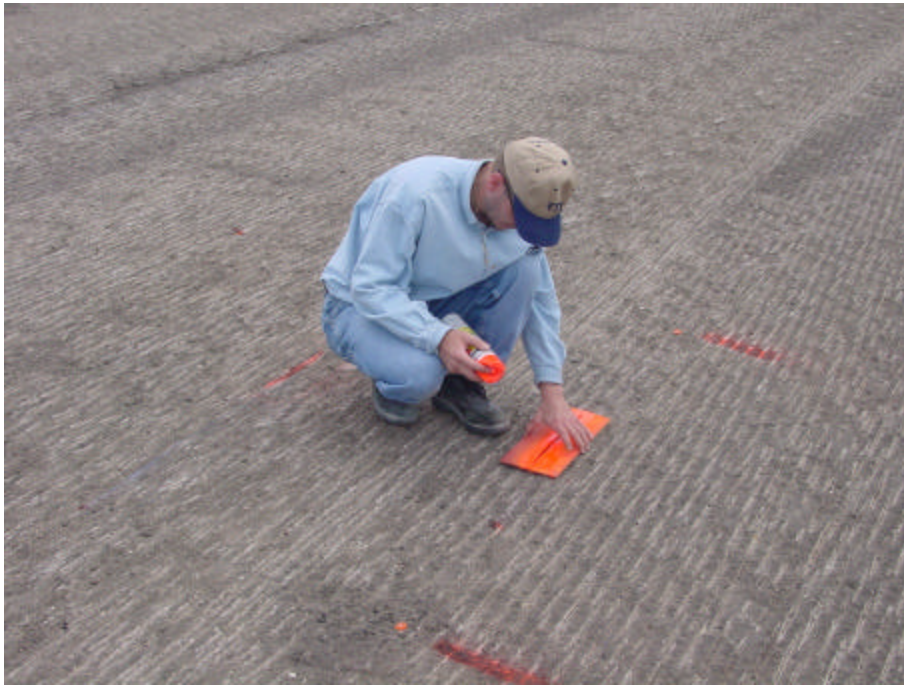
Figure 10 Identification and Marking of Test Slab and Gage Locations
