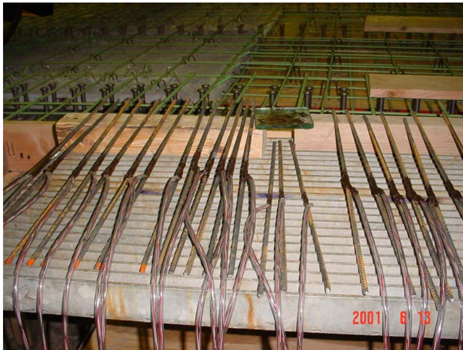
Figure 5.13 – Bars with Strain Gages
