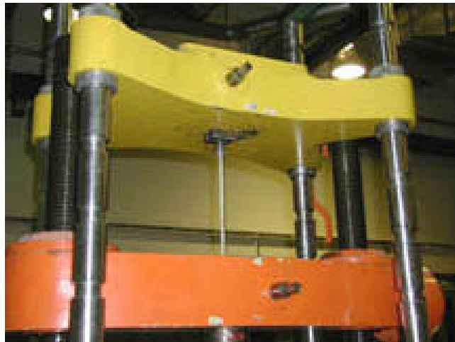
Figure 17: 24-Inch FRP Bar in Tensile Testing Apparatus
