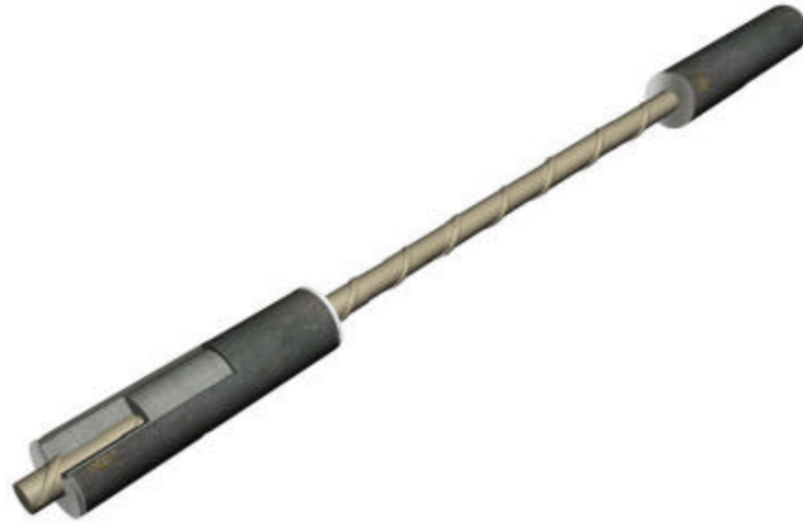
Figure 9: 3-D View of Bar and Anchor Layout
