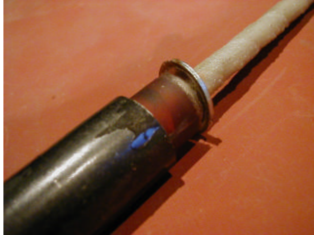
Figure 10: Bar and Epoxy Pullout
