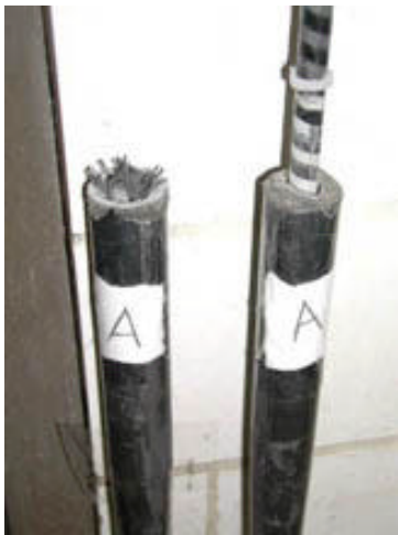
Figure 21: Uncond. CFRP Failure
