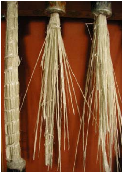
Figure 3.5 - Failure Mode of 1/2" GFRP R
