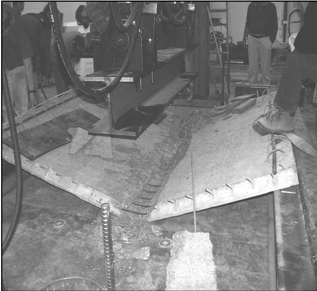
Figure 4.11 - CDOT Panel Failure
