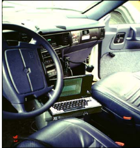
Figure A-1 Mobile Data Terminal
