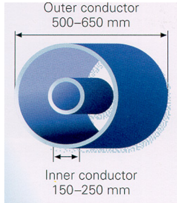
Figure 54: Cross Section of Siemens GIL
