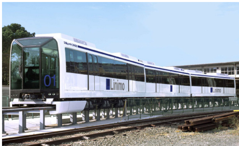
Figure 85: HSST Linimo maglev vehicles for the Tobu Kyuryo Line in Nagoya, Japan
