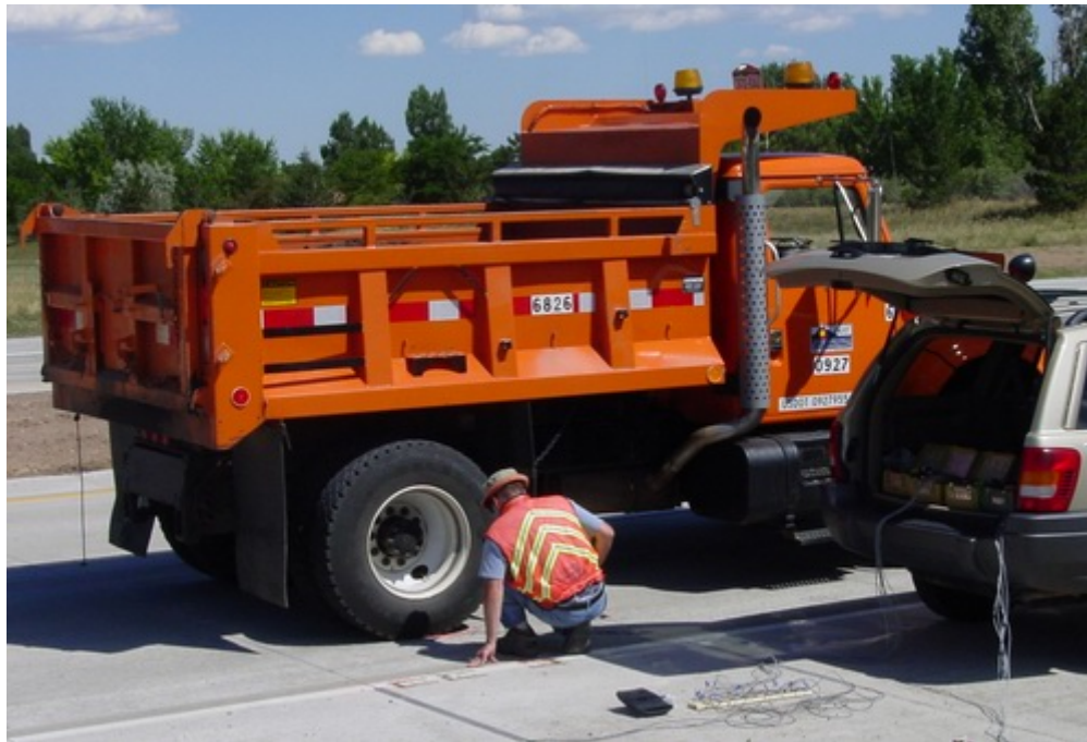
Figure 4.3. Truck Wheel Placement During Load Testing
