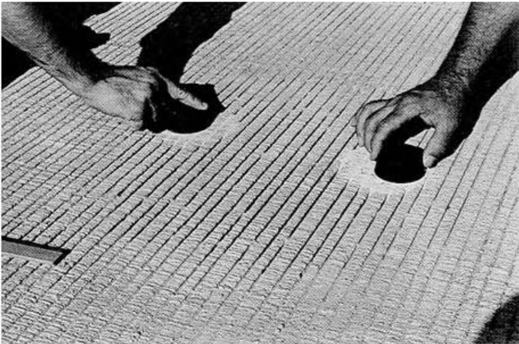
Photo 22: Sand patch test for measuring texture depth
