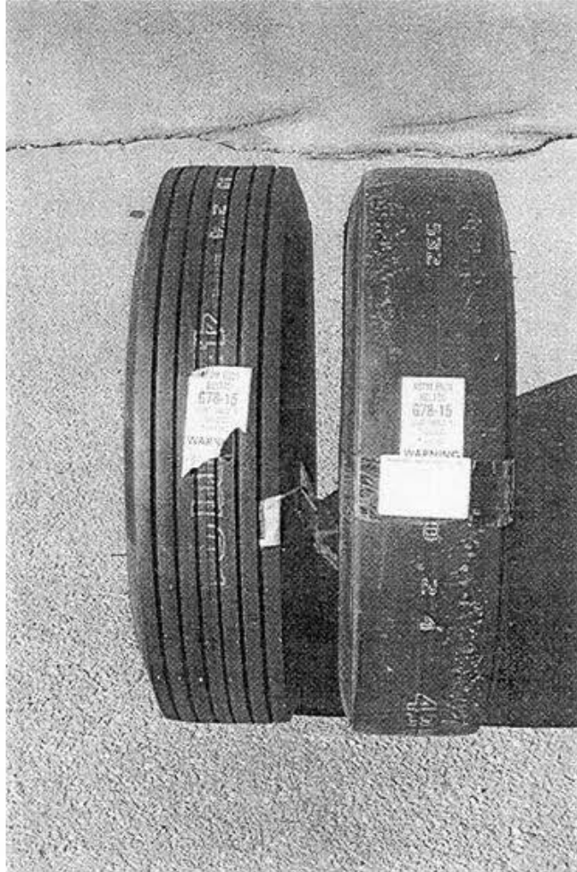
Photo 1: View of the ribbed tire (ASTM E 501 and The smooth tire (ASTM E524)
