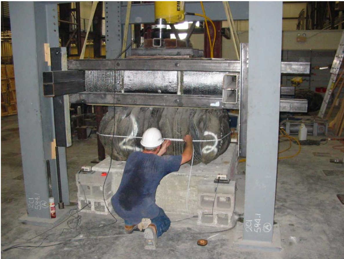
Figure 6: Circumferential measurements. Outriggers mitigated rotation problem.
