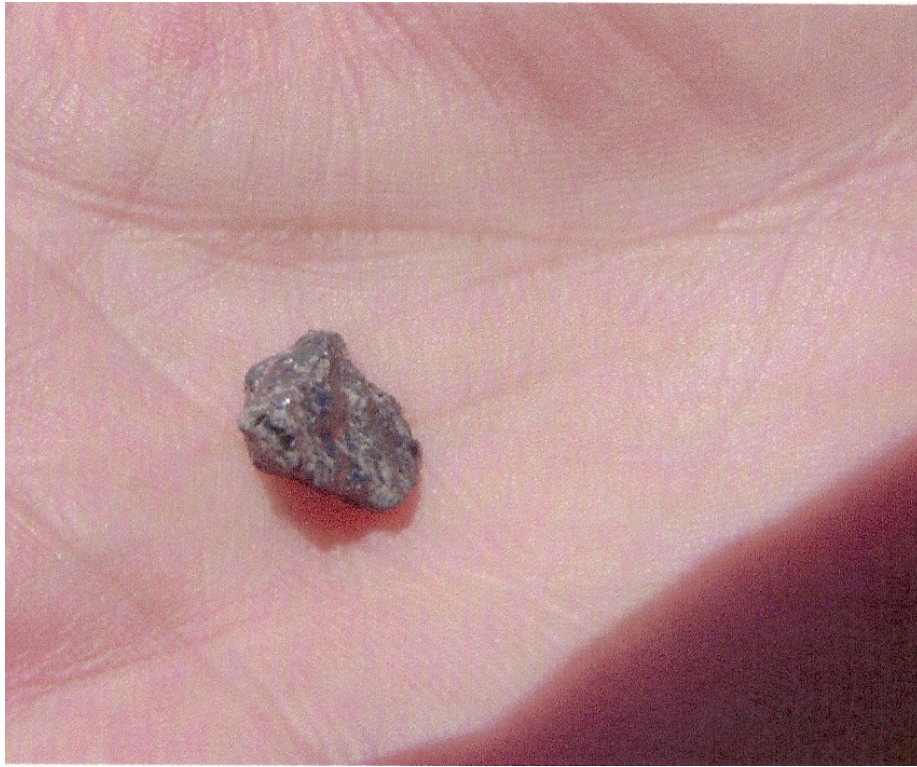
Figure 2. Large Steel Slag Aggregate, Note Angularity and Rough Surface Texture
