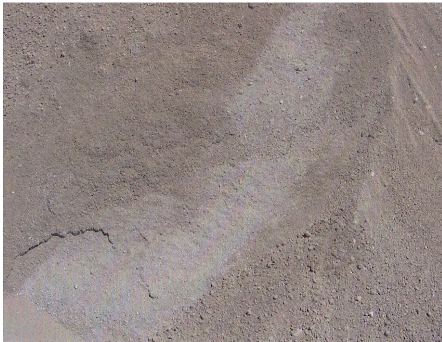
Figure 3. Steel Slag Aggregate Stockpile
