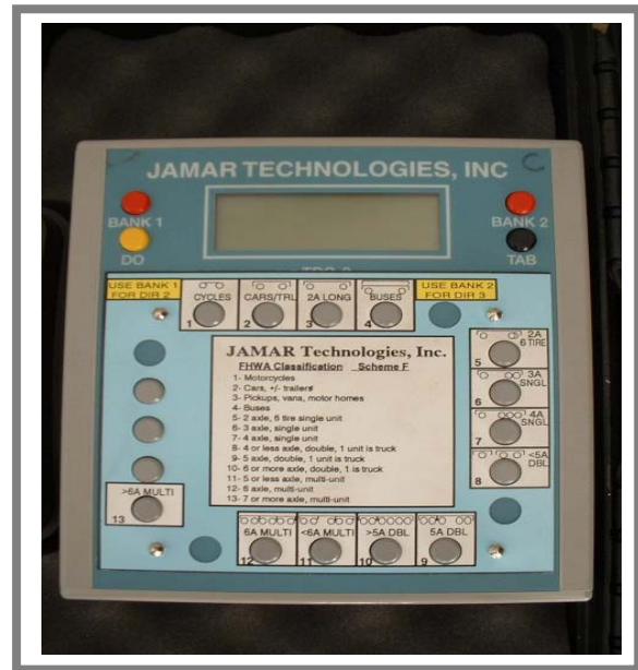
Figure 2: Example Count Board with FHWA 13-Bin Classification Template
