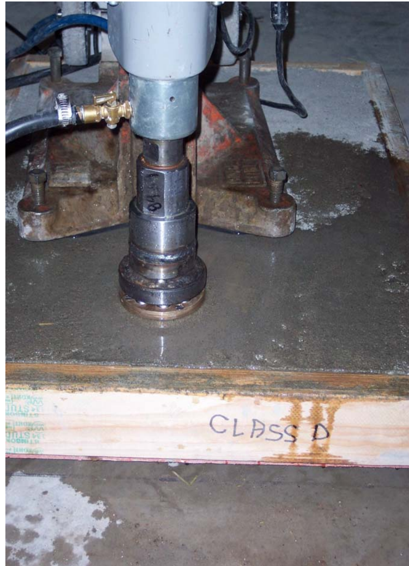
Close-up of custom designed abrasion attachment
