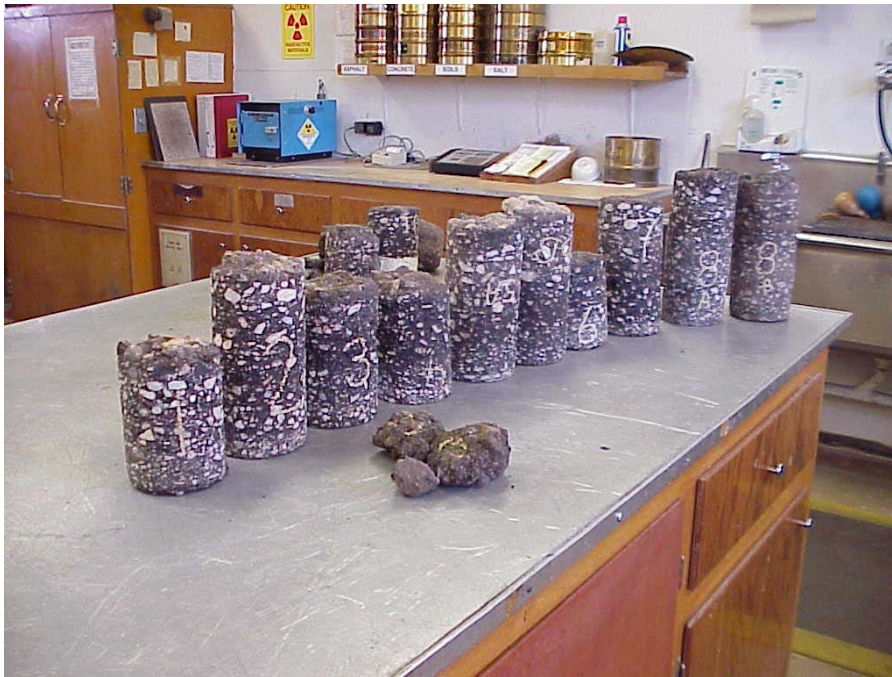
Figure 13: Coring samples 9 through 19 taken for 2001 rehabilitation
