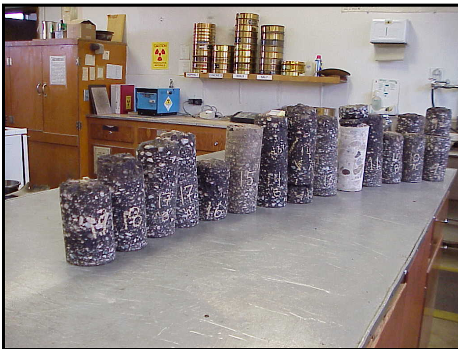
Figure 13: Coring samples 9 through 19 taken for 2001 rehabilitation
