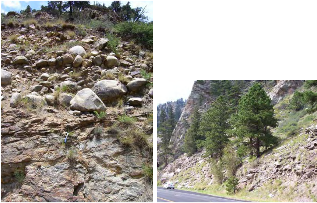
Figure 2.27: Block-in-matrix block shape: Picture on left was taken on I-70 in Clear Creek County. The slope contained several rounded blocks (score of 81). Picture on right was taken on U.S. 34 in Larimer County. The slope contained tabular blocks of mica schist (score of 3).
