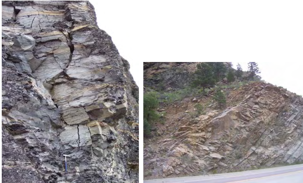
Figure 2.23: Discontinuity aperture: Picture on left was taken on CO 9 in Summit County. The discontinuities had an aperture of > 5 mm (score of 81). Picture on right was taken on U.S. 6 in Clear Creek County. The discontinuities had an aperture of 0.1 – 1 mm (score of 9).
