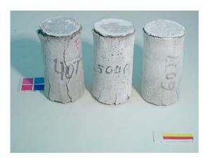
Figure 5.3. Cylinders exposed to CaCl<sub>2</sub> solution after 84 days of constant low temperature test. From left to right: 0.40, 0.50, and 0.60 *w/c* mortar cylinders.
