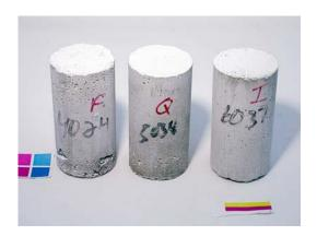
Figure 5.27. Cylinders exposed to 10% CaCl<sub>2</sub> solution after 56 days of constant low temperature test.
