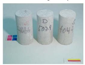
Figure 5.1. Cylinders exposed to NaCl solution after 84 days of constant low temperature test. From left to right: 0.40, 0.50, and 0.60 *w/c* mortar cylinders.
