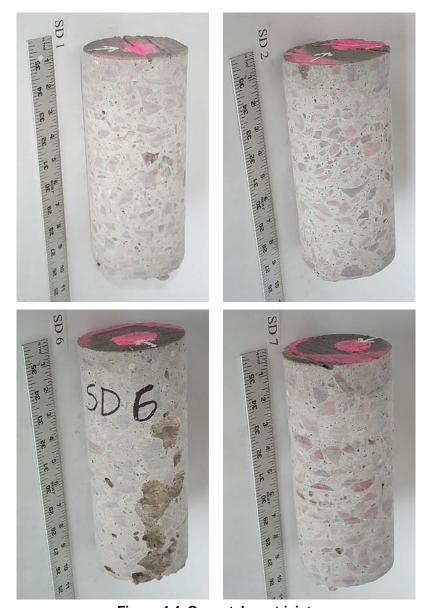
Figure 4.4. Cores taken at joint.
