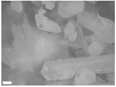
Figure 5.70. CaCl<sub>2</sub>•Ca(OH)<sub>2</sub>•2H<sub>2</sub>O crystals before, (top) and after immersion in distilled water in atmospheric equilibrium with CO<sub>2</sub> at room temperature and subsequent alteration.
