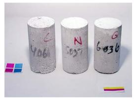
Figure 5.25. Cylinders exposed to 3% CaCl<sub>2</sub> solution after 56 days of constant low temperature test.
