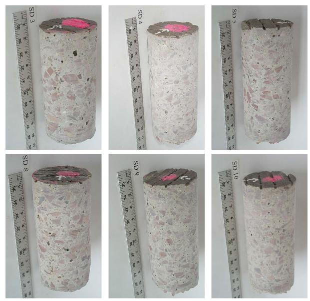
Figure 4.4. Cores taken away from joint.
