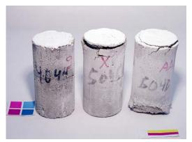
Figure 5.29. Cylinders exposed to 17% CaCl<sub>2</sub> solution after 56 days of constant low temperature test.
