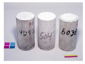
Figure 5.28. Cylinders exposed to 14% CaCl<sub>2</sub> solution after 56 days of constant low temperature test.
