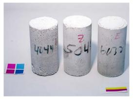
Figure 5.26. Cylinders exposed to 7% CaCl<sub>2</sub> solution after 56 days of constant low temperature test.
