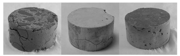
Figure 5.50. Photographs of 4 inch [100 mm] diameter 0.45 w/c ordinary portland cement (OPC) concrete specimens after 500 days in high concentration brines.
