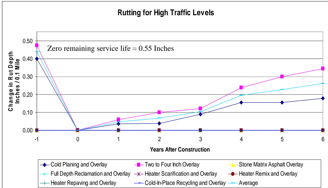
Figure 24 Permanent deformation performance after six years with relation to traffic counts from 3 to 11 million ESAL
