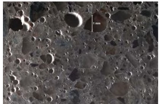
Magnification: 10x Description: Hardened air void system.
