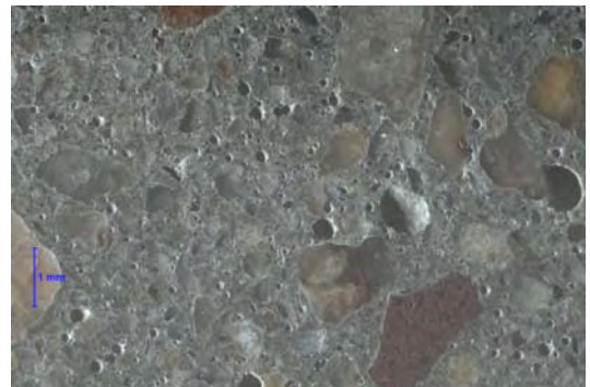
Magnification: 15x Description: Hardened air void system.
