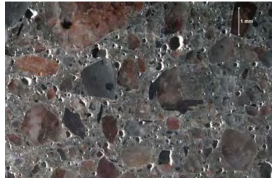
Magnification: 10x Description: Hardened air void system.
