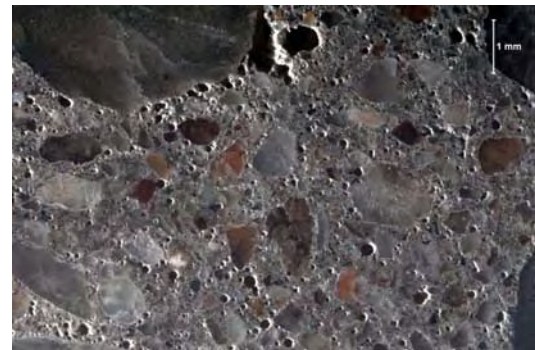
Magnification: 10x Description: Hardened air void system.
