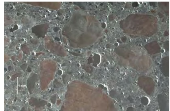
Magnification: 15x Description: Hardened air void system.
