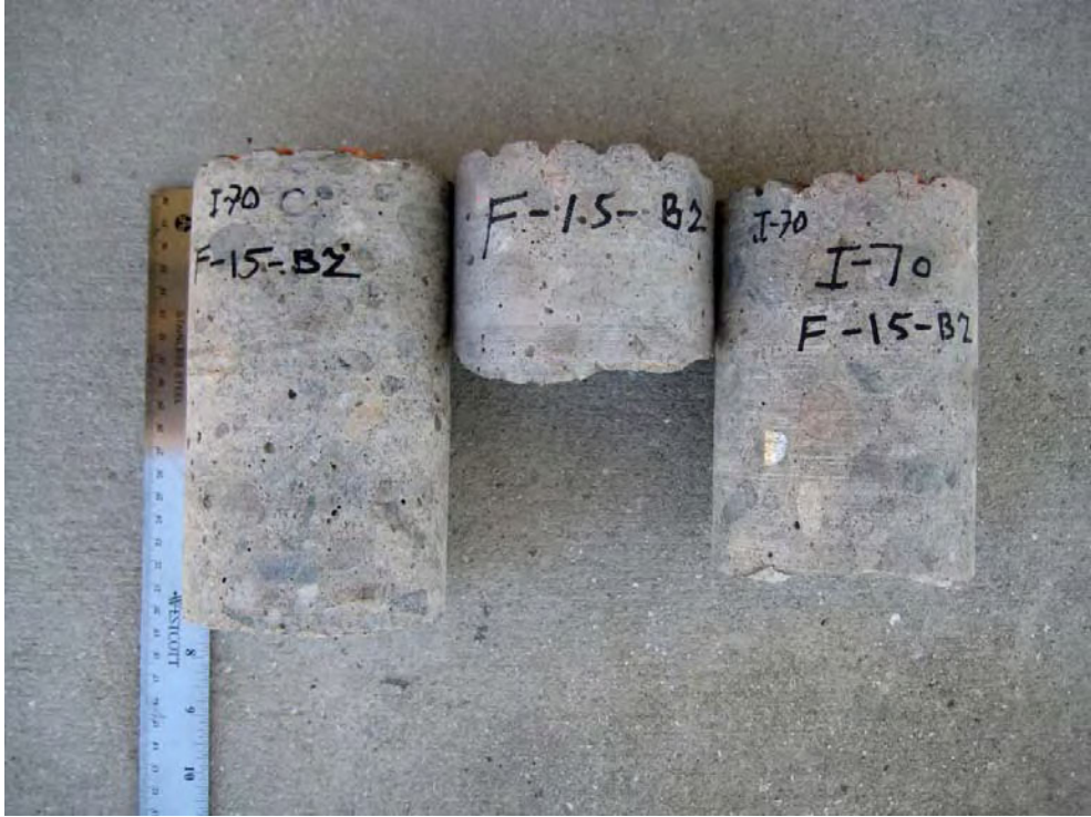
Figure 18. Core samples received by the laboratory for Structure F-15-BZ
