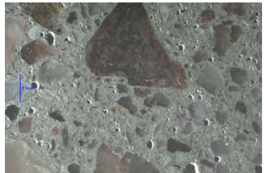
Magnification: 15x Description: Hardened air void system.
