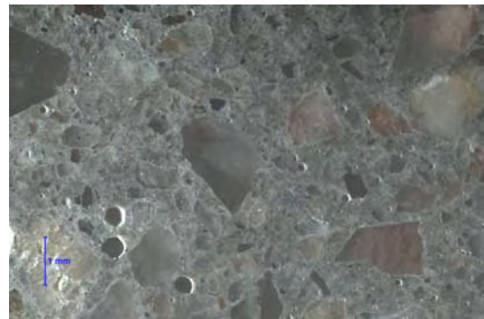
Magnification: 15x Description: Hardened air void system.
