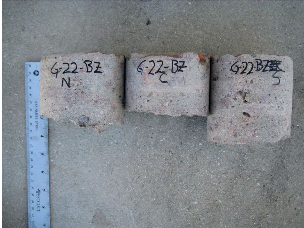
Figure 20. Core samples received by the laboratory for Structure G-22-BZ
