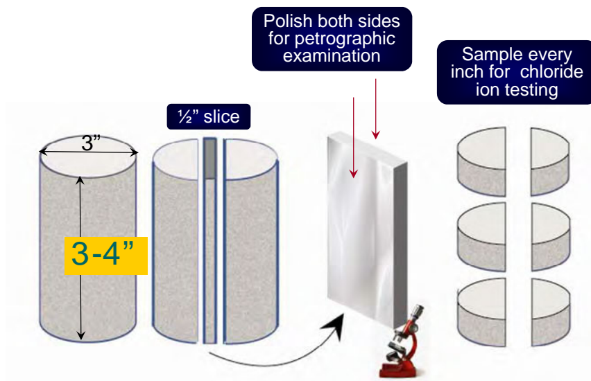
Figure 21. Samples obtained from each core for petrographic and chloride testing
