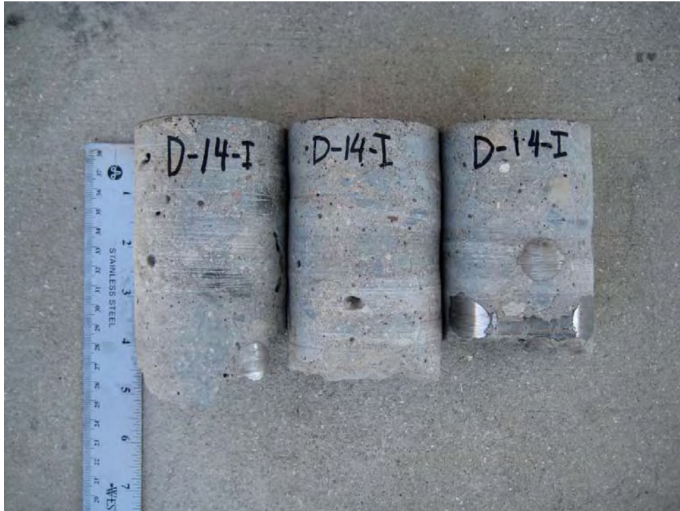
Figure 16. Core samples received by the laboratory for Structure D-14-1
