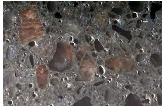
Magnification: 10x Description: Hardened air void system.
