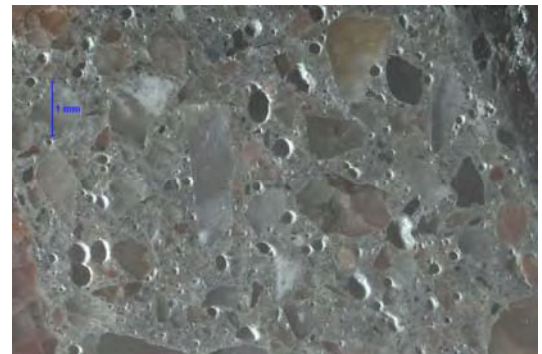
Magnification: 15x Description: Hardened air void system.
