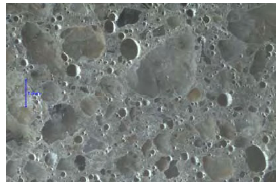
Magnification: 15x Description: Hardened air void system.
