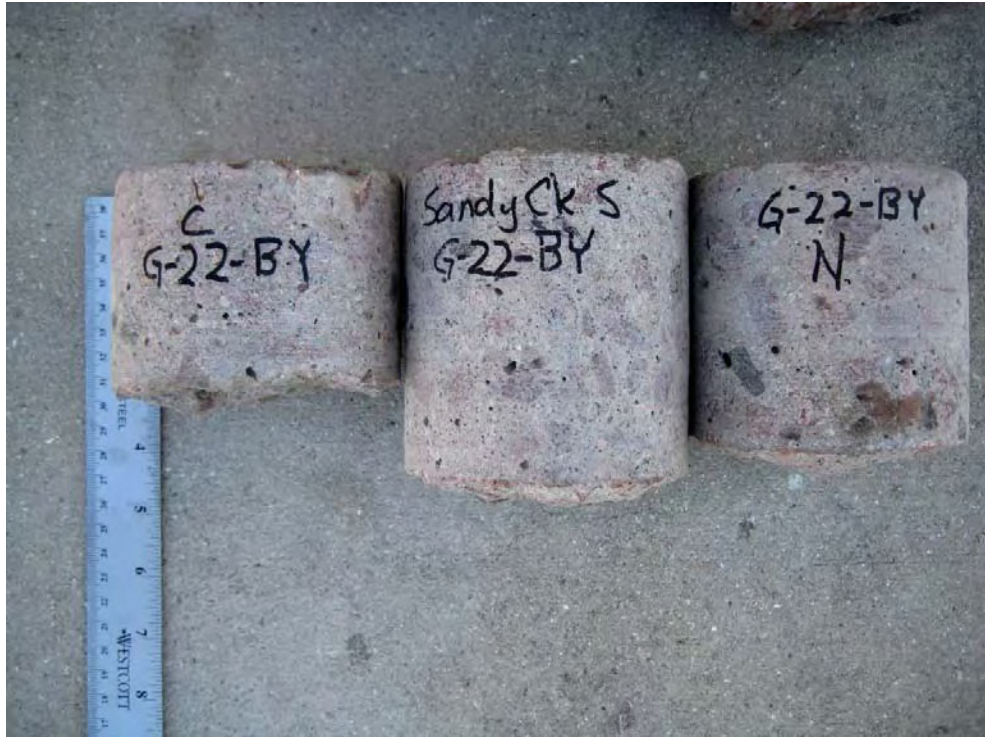
Figure 19. Core samples received by the laboratory for Structure G-22-BY
