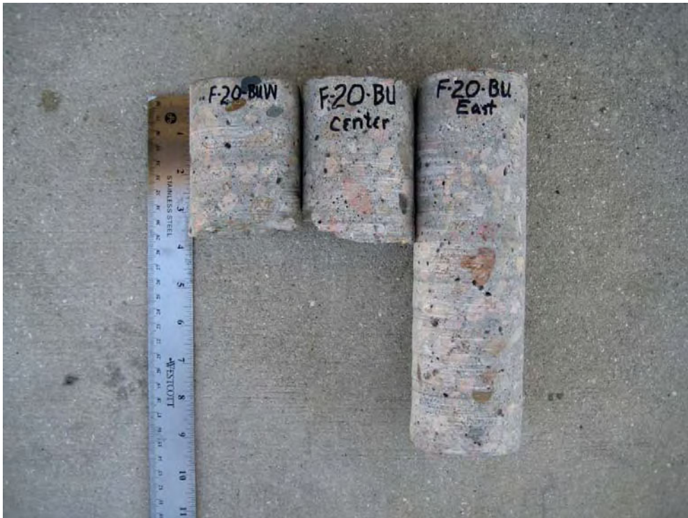
Figure 17. Core samples received by the laboratory for Structure F-20-BU
