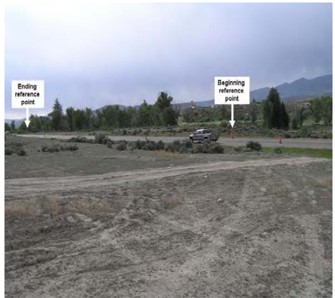
Figure 4. The white car to the left cleared the reference area before the pickup entered. The pickup is counted.
