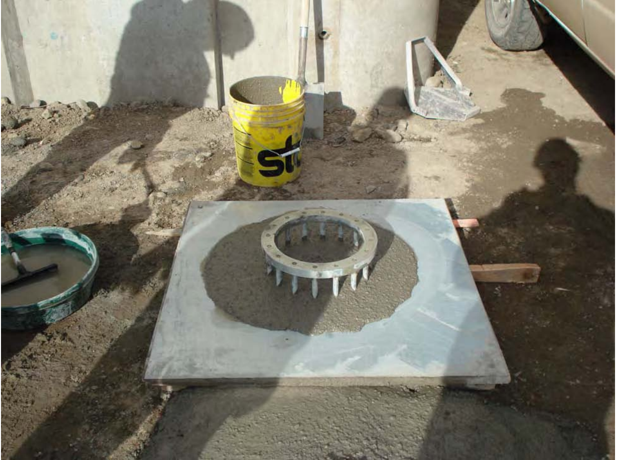
Figure 2: Slump Flow Through J-Ring
