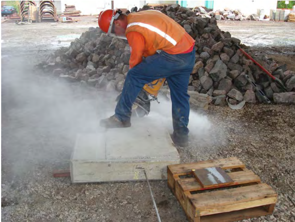
Figure 7: Saw Cutting of Specimens
