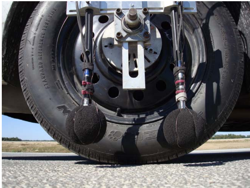
Figure A.1. OBSI Measurement Bracket Configuration.
