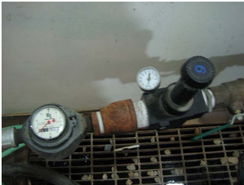
Figure 5. Pressure regulator and flow meter to measure inflow into the rainfall simulator.
