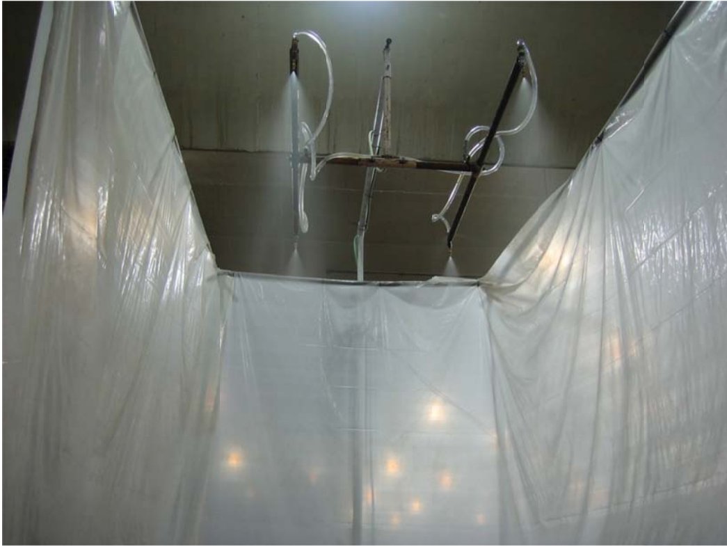
Figure 4. The rainfall simulator with 4 spray nozzles.
