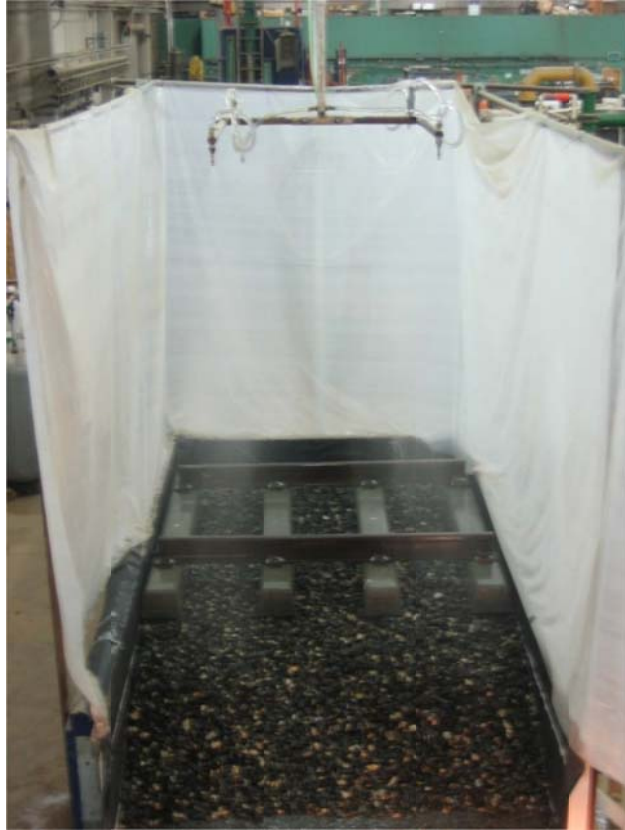
Figure 2. The overall model during a rainfall simulation event.
