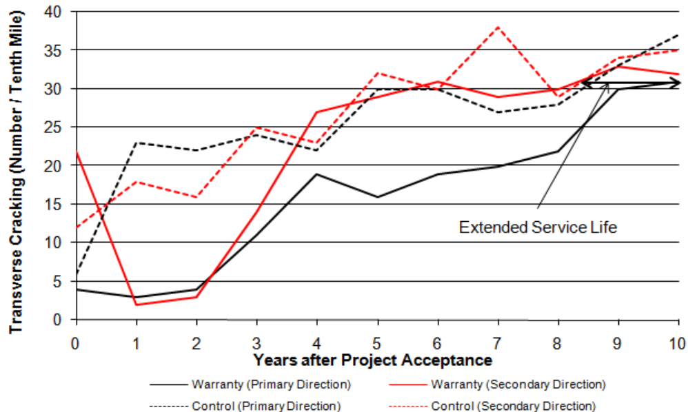
Figure 26. Comparison of the US 36 / I-76 transverse cracking performance
