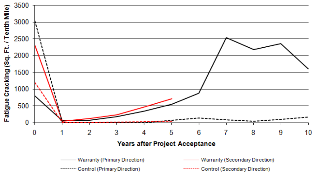
Figure 66. Comparison of the US 36 East of Byers/US 36 West of Byers fatigue cracking performance
