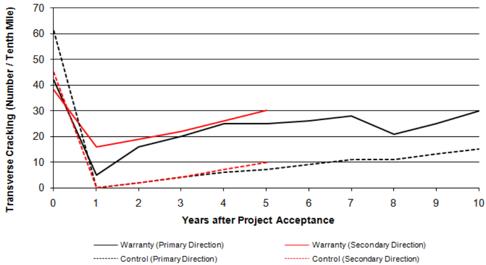
Figure 68. Comparison of US 36 East of Byers/US 36 West of Byers transverse cracking performance
