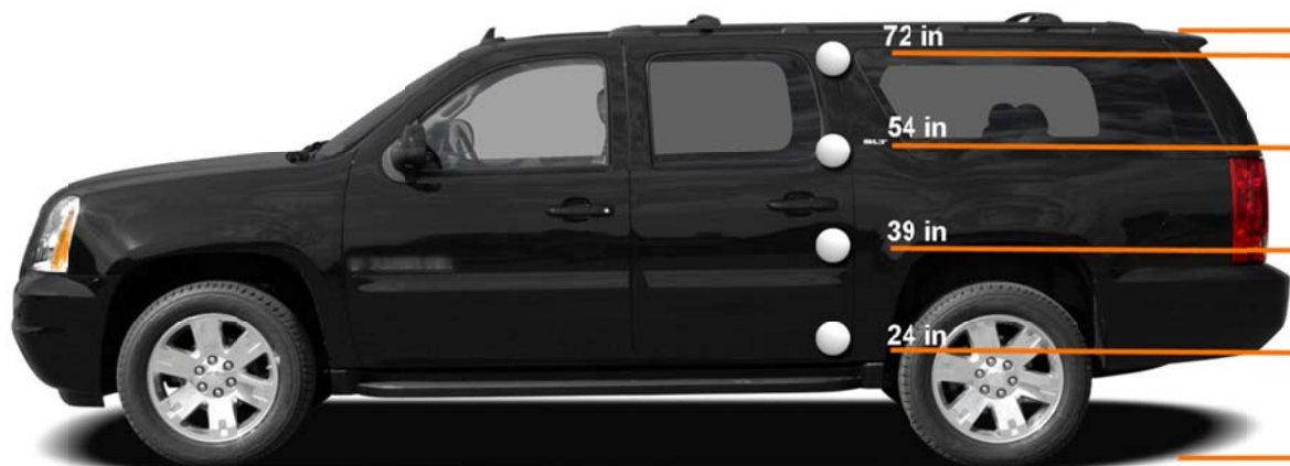
Figure 6: Light meter orientation, vehicle side.
