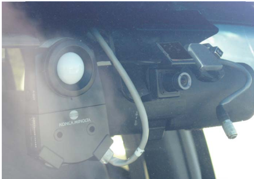
Figure 11: Glare meter inside front windshield.
