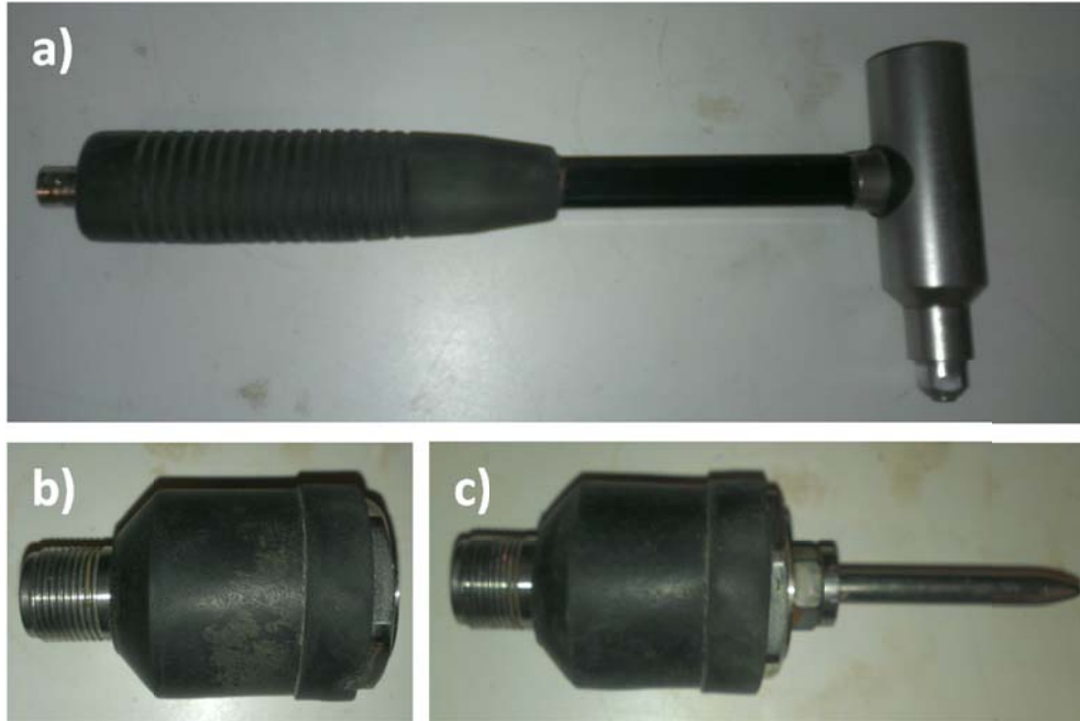
Figure 5.4: (a) instrumented hammer used as source impact, (b) accelerometer with no spike for greased coupling, and (c) accelerometer with ground spike for direct coupling.
