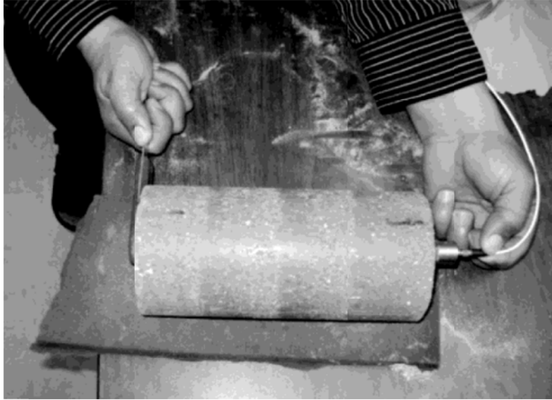
Figure 5.3: Free-free resonance testing with longitudinal excitation.
