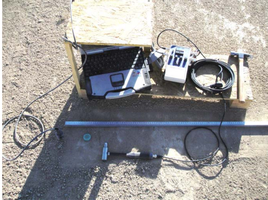
Figure 3.11: SeisNDT experimental surface wave test setup.
