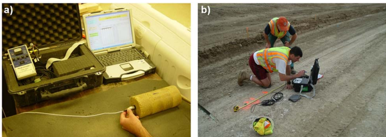
Figure 2.3: (a) SeisNDT experimental setup for free-free resonance and (b) surface wave testing.
