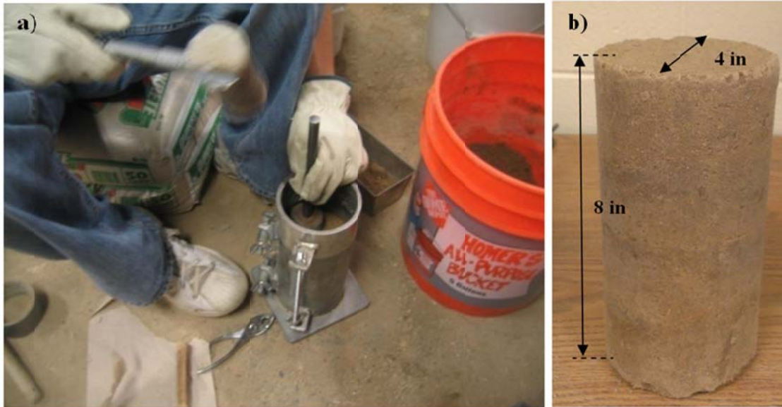
Figure 5.1: (a) FFR cylinder preparation and (b) example cylinder.
