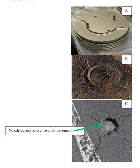
Figure 9: Spray nozzles used for mounting in the pavement A) Stainless steel nozzle B) Rubber and stainless steel nozzle C) Buried nozzle in asphalt pavement
