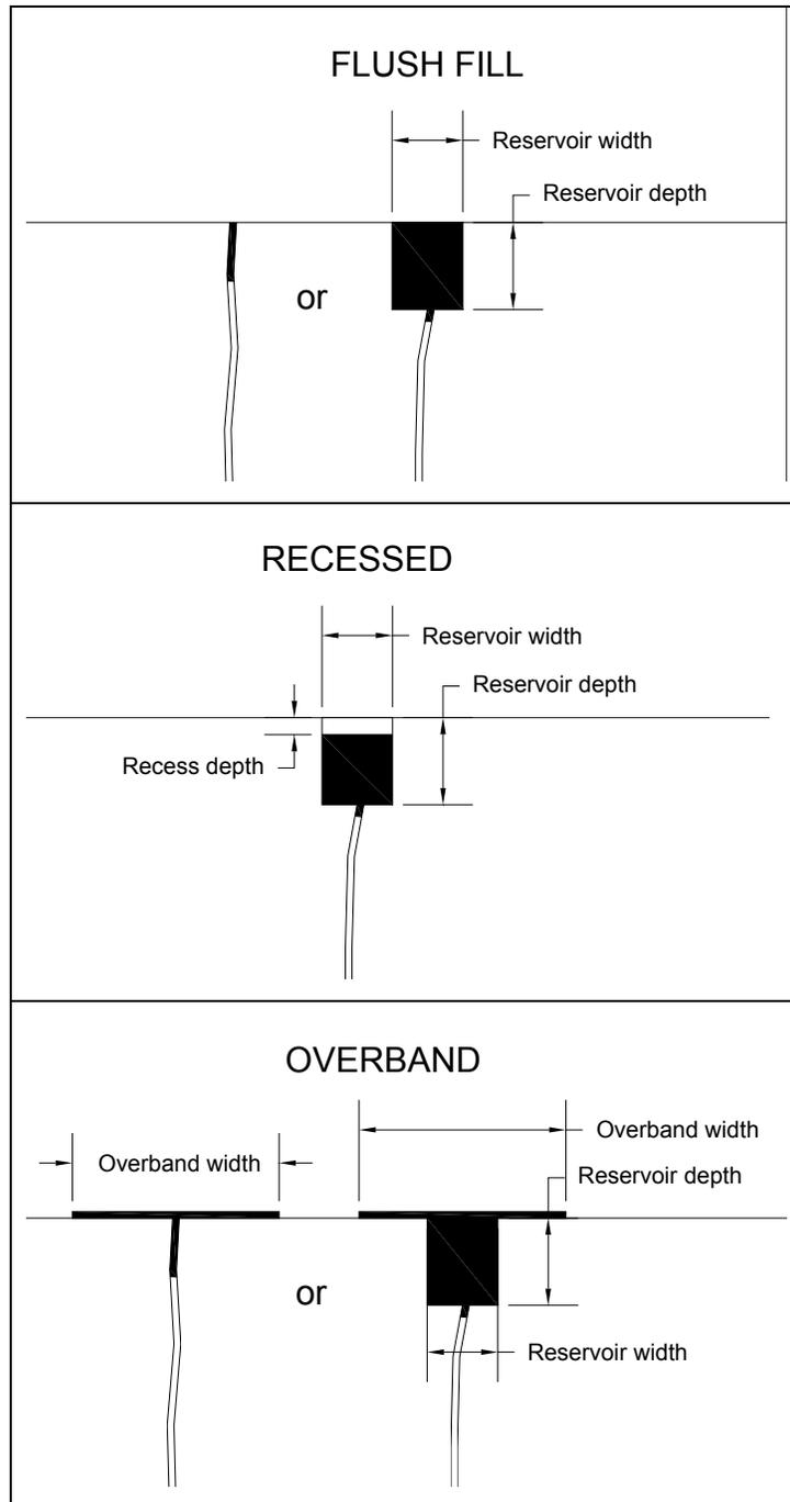
Figure 12. Crack sealing and filling configurations.
