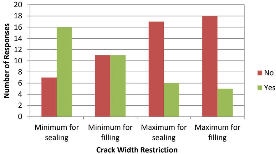
Figure 2. Policy restrictions on crack width for filling and sealing from survey responses.
