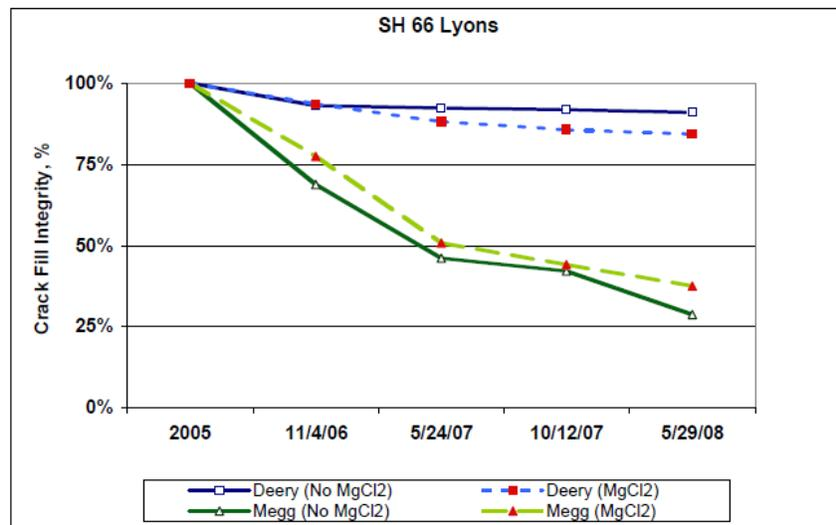
Figure 17. Crack seal effectiveness over time at SH 66 Lyons (Shuler 2010).
