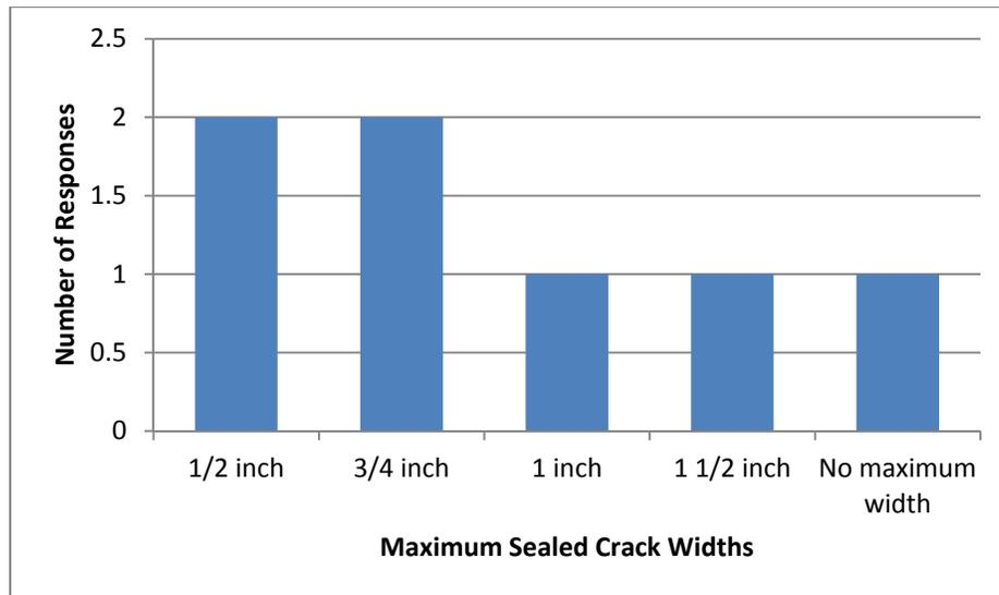
Figure 6. Maximum crack widths for sealing identified by CDOT respondents.
