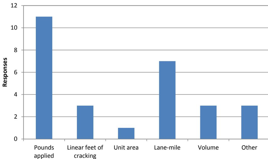
Figure 11. Survey responses on crack sealing or filling bid methods.
