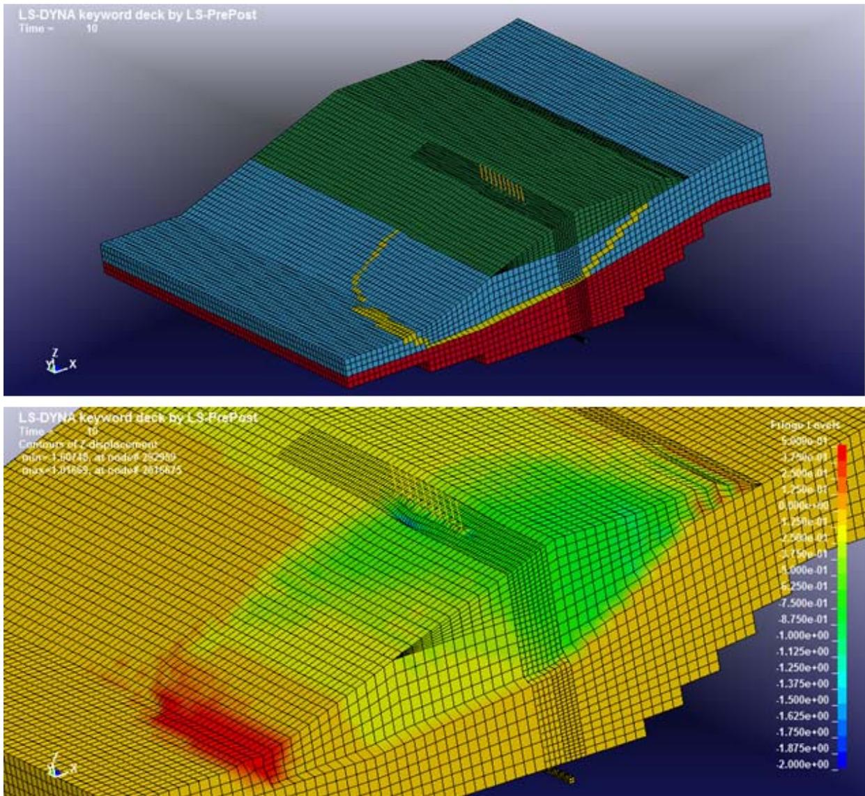
**Figure 7: Mitigated slope with the use of driven piles at the failure edges and contours of vertical deformation**
