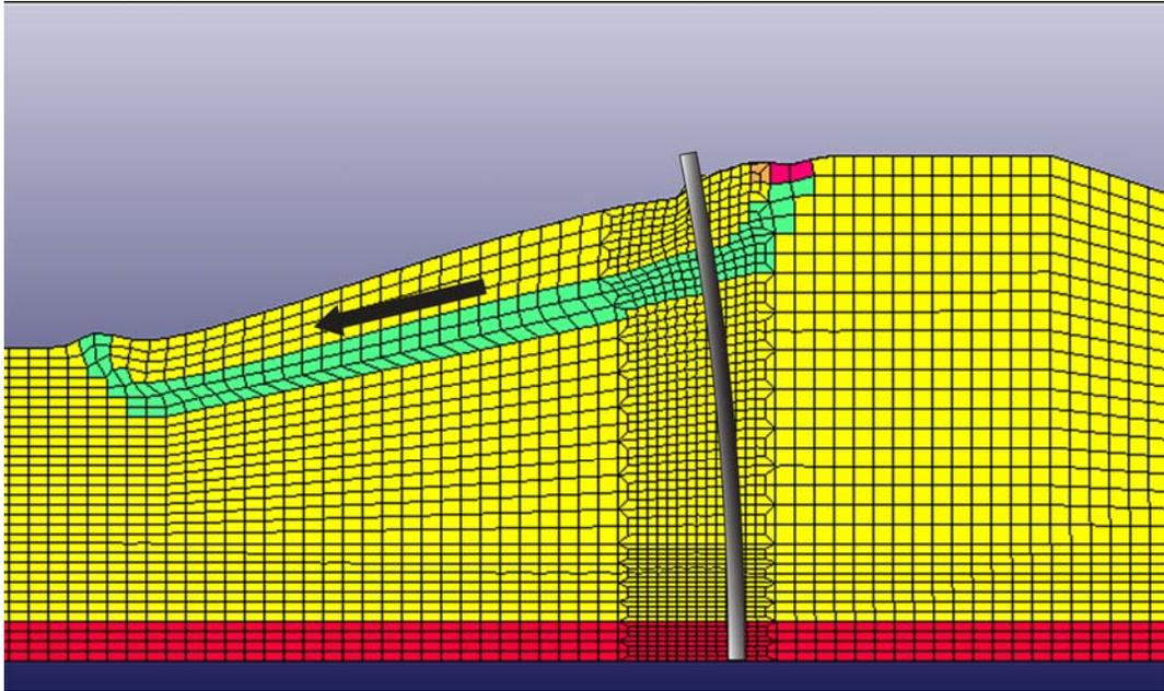
**Figure 17: Deformed pile in 3:1 slope with shallow failure**
