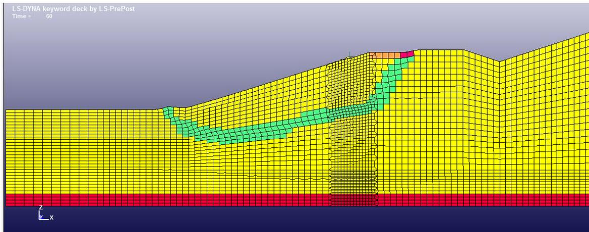
(B): Mitigation based on HP 14x102 driven piles spaced at 5 ft.
