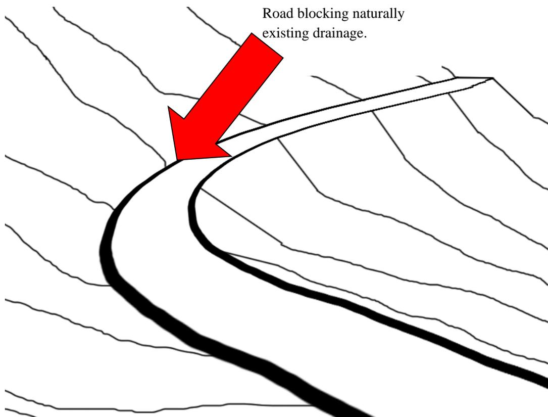
**Figure 3. Naturally existing drainage blocked by road.**
