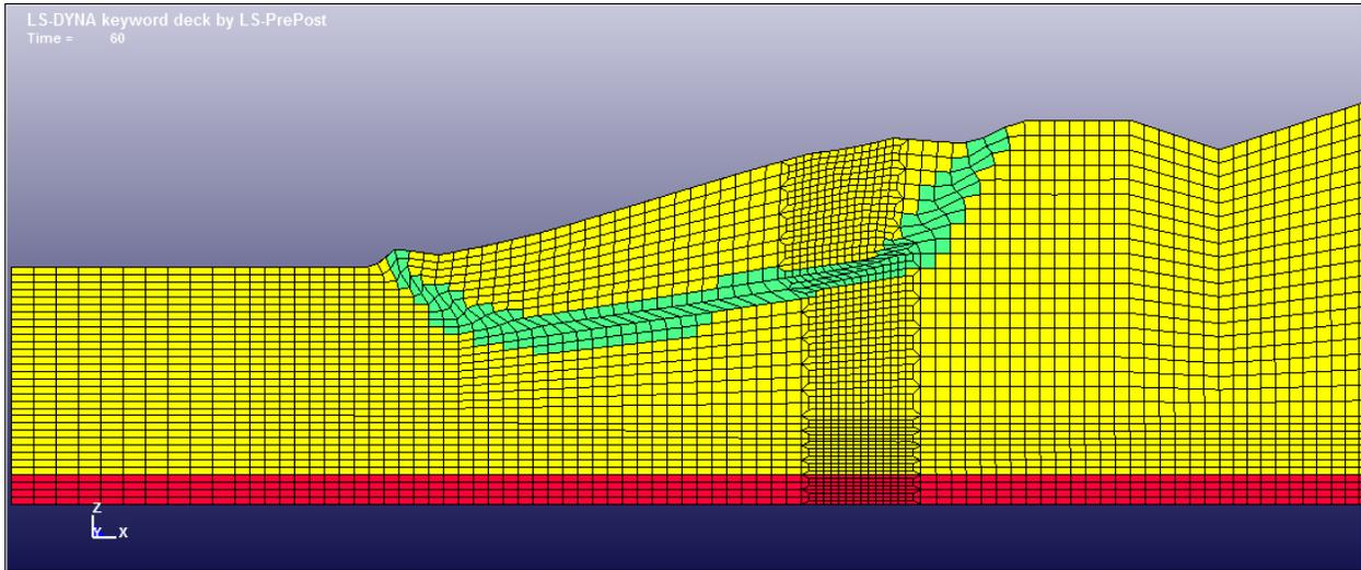
(A): Unmitigated failure of a 3:1 slope embankment
