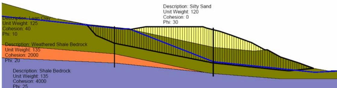
Figure 5: Soil stratification of the Muddy Pass Slide
