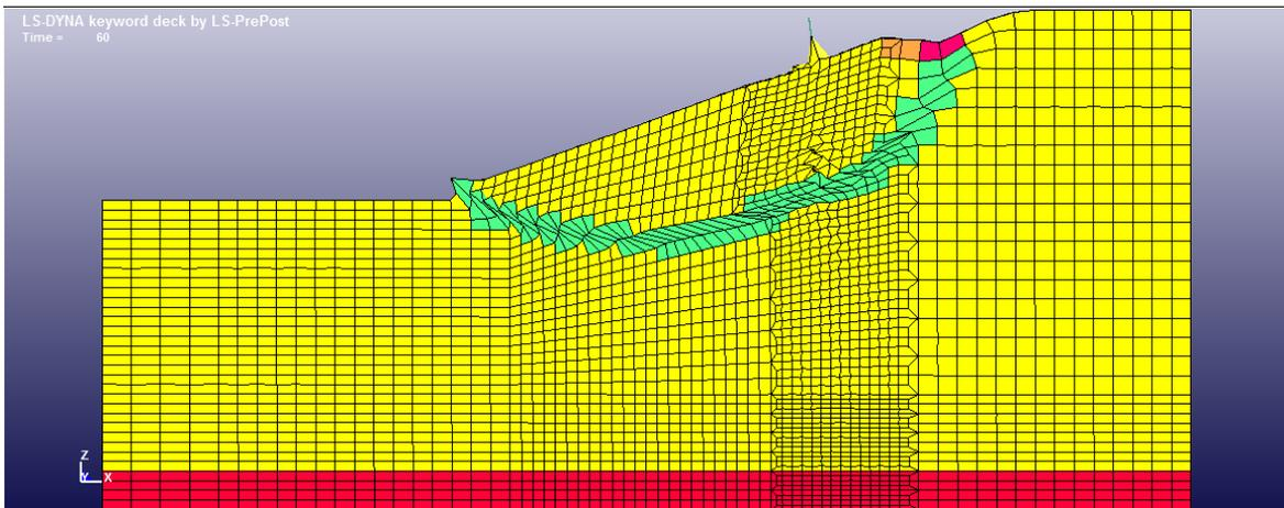
(C): Mitigation based on HP 18x204 driven piles spaced at 5 ft.
