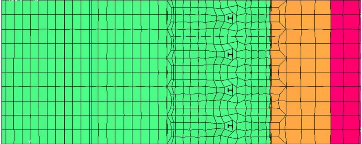
**Figure 19: Soil flow between driven piles**
