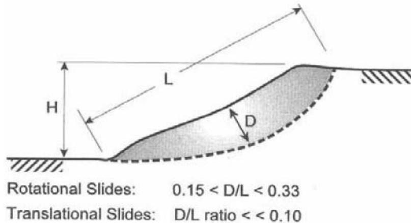
**Figure 2. Aspect ratio of failure mass (Abramson et al., 2002).**
