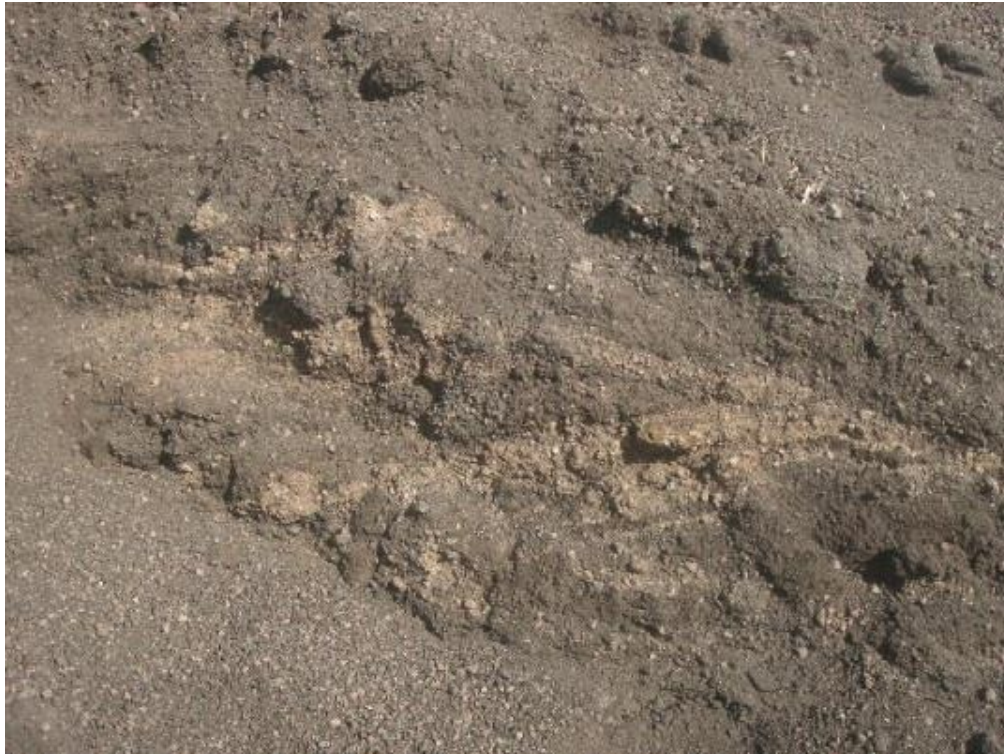
Figure 2. Topsoil mixed with subsoil.
