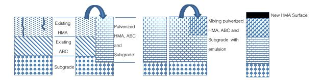
Figure 6. Typical Sequence of an AEFDR Process
