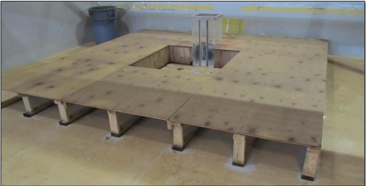
*Figure 38. Model setup for horizontal grate testing.*
