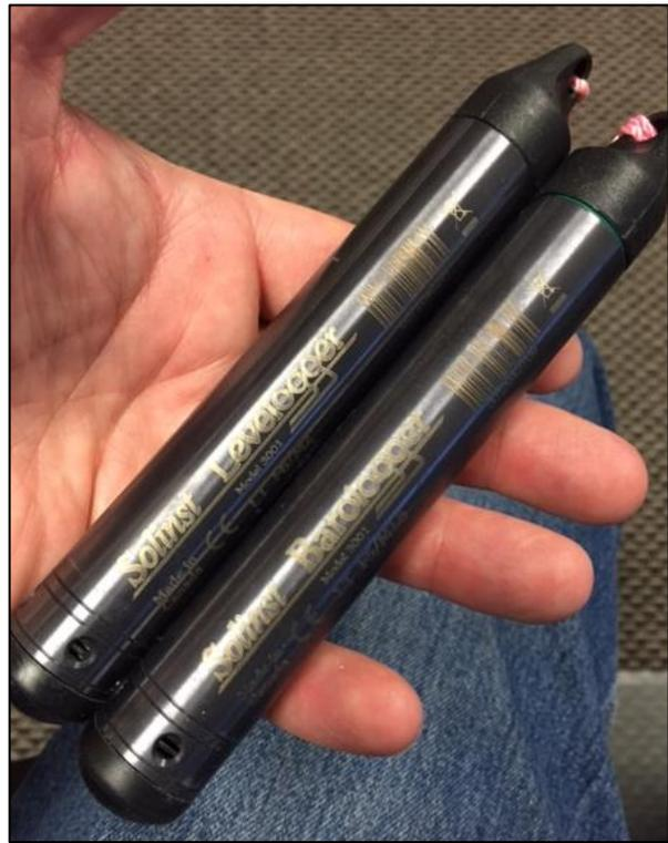
Figure 17. Levelogger™ pressure transducer installation over 2014 and 2015 rainfall seasons allowed testing of the elliptical slot weir in the field.
