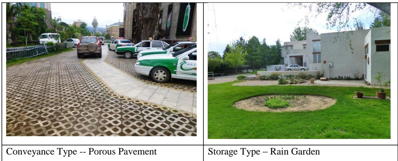
**Figure 1.2 Conveyance and Storage Low-Impact Designs**
