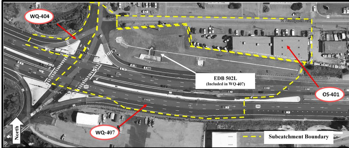
**Figure 2.7 Tributary Sub-catchments to WQB in EDB 502L**
