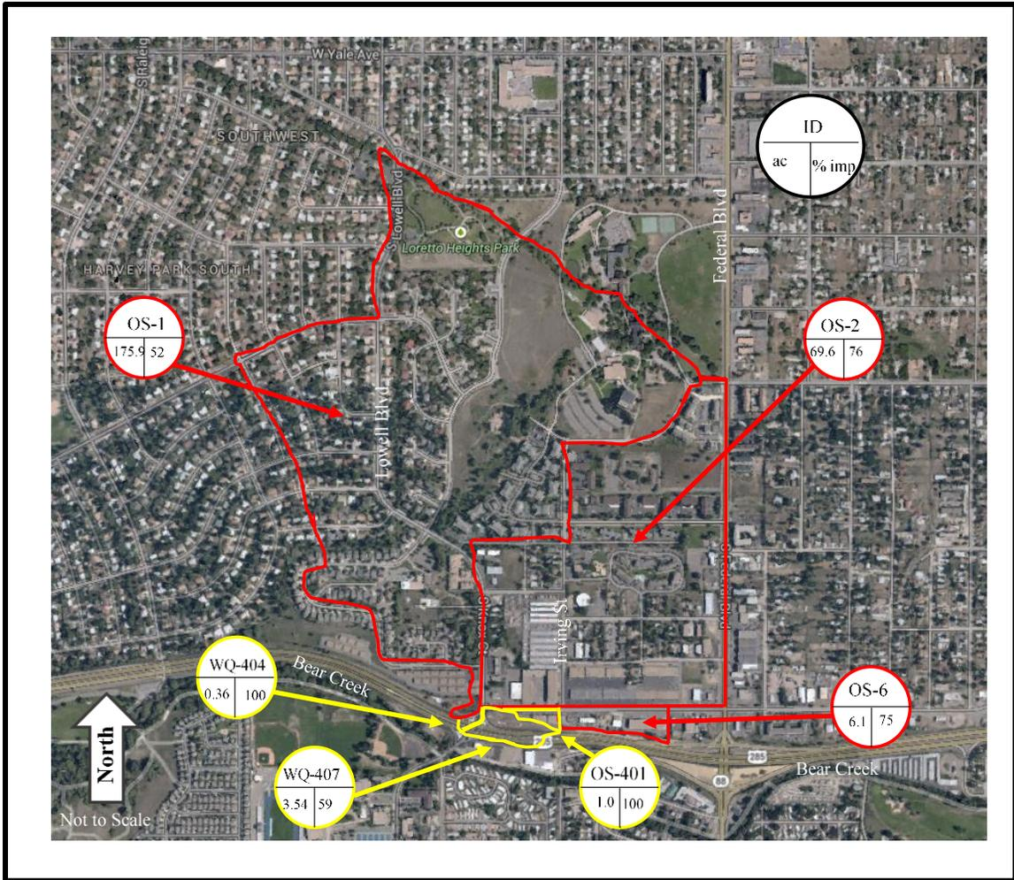
**Figure 2.8 Off-site Sub-catchments Tributary into EDB 502L**
