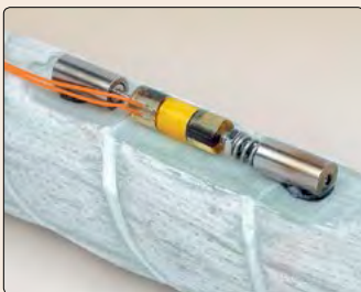
● Model 4151 Strain Gage mounted to a fiberglass rebar.
