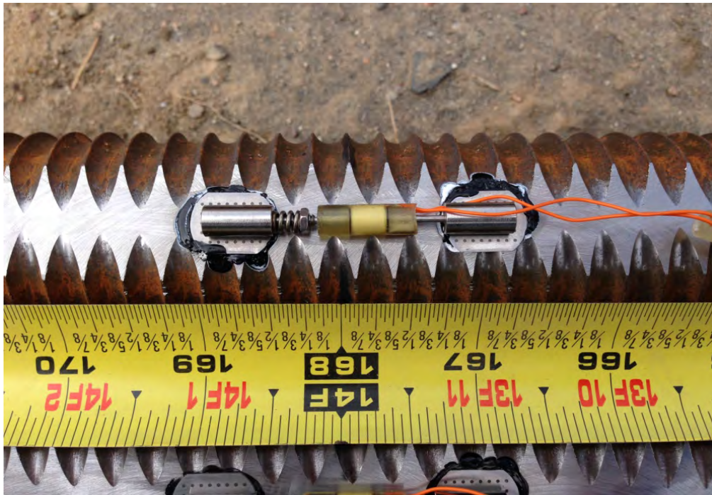
Photograph A-4. Tie-Rod Strain Gage.
