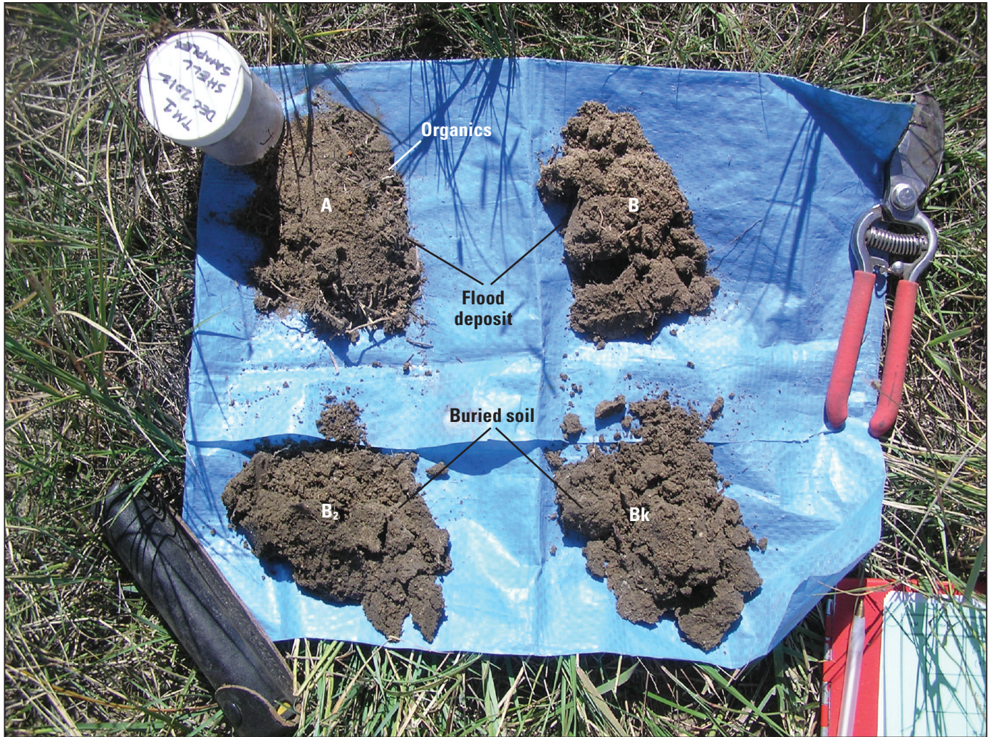
Figure 1-4. These soil samples correspond to the soil horizons in figure 1-3. The soil structure goes from single grained and weakly granular in the A horizon to weak to moderate subangular blocky in the B k horizon. Photograph by Jeanne Godaire, Bureau of Reclamation.
