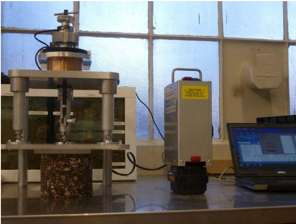
**Figure 3. Direct Tension Core in Position for Testing**
