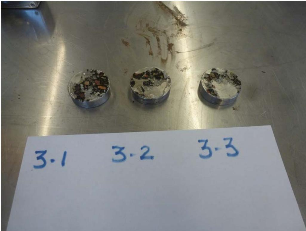
**Figure 5. Direct Tension Core Failure at Grip**
