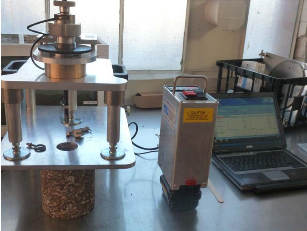
**Figure 2. Direct Tension Apparatus**
