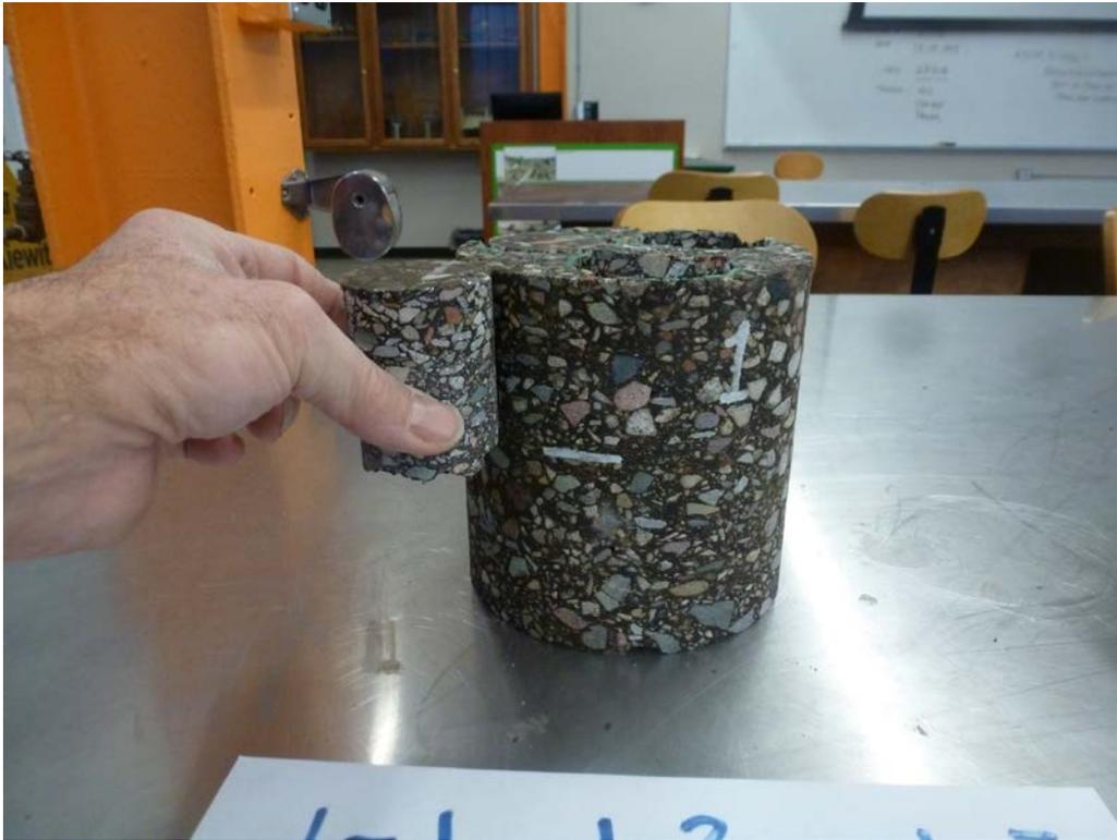
**Figure 4. Direct Tension Core Failure at Interface**
