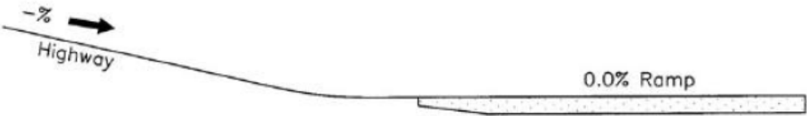
Figure 1.5. Horizontal Grade EER Reprinted from AASHTO’s Green Book (p. 144), by the American Association of State Highway and Transportation Officials, 2011, Washington DC.
