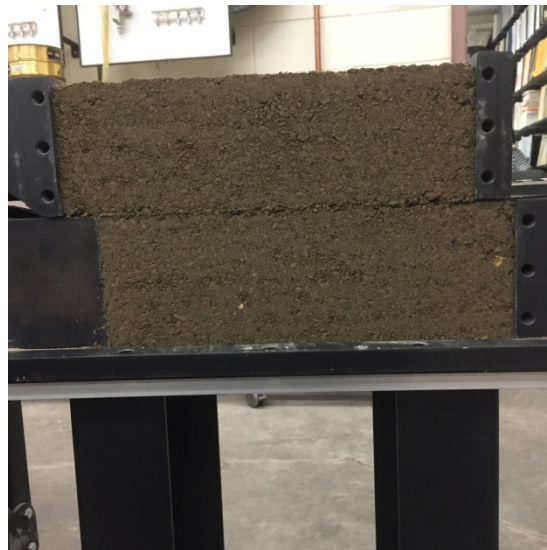
Figure 25. Backfill with geosynthetic inclusion after shearing
