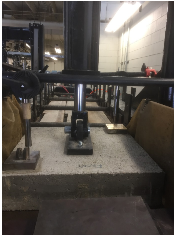
Figure 43. Install the loading plate, vertical displacement sensors, and airbag
