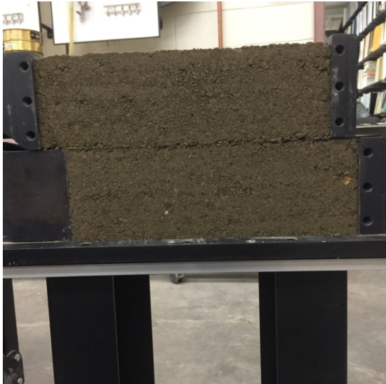
Figure 46. Backfill with geosynthetic inclusion after shearing
