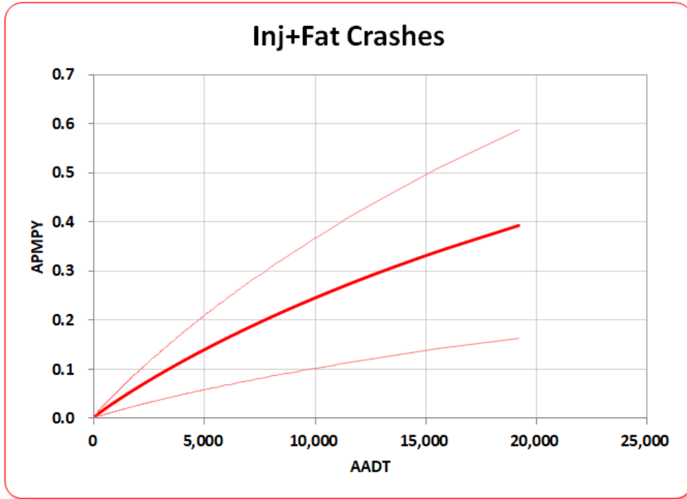
Figure 63. SPF - Rural Flat and Rolling 2-Lane Highways – Fixed Object Collisions – Severity Model
